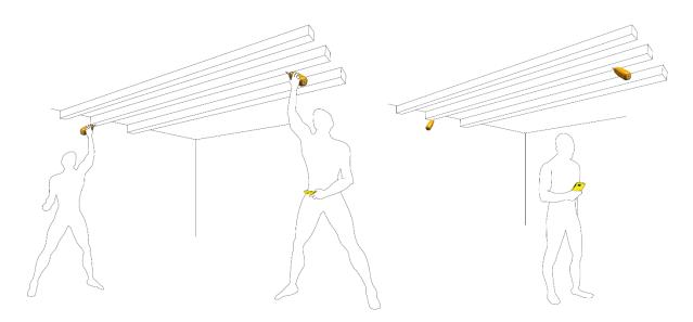
The indirect mode is used, for example, in building surveys when the ends of the wood are not accessible for direct measurements.
