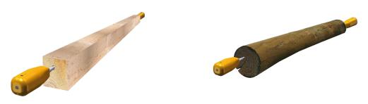
To evaluate the mechanical properties of structural wood, longitudinal measurements in direct mode are to be preferred.
